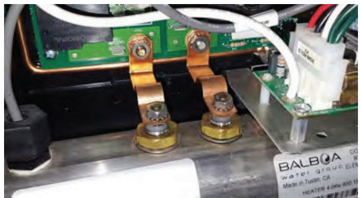
Close-up of the two copper straps that connect the heater to the spa pack circuit board.
